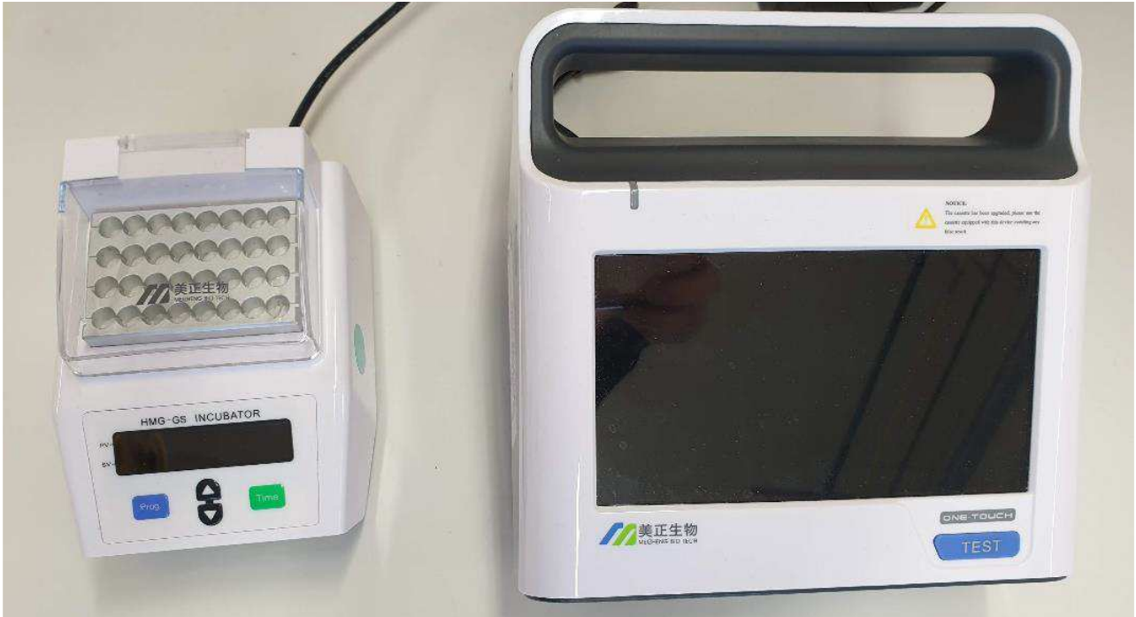
Fig. 2. HMG-GS Microwell Incubator and BMZ6000 Portable Strip Reader for instrumental reading of the color formation on the AnticFast® Beta-lactams & Tetracyclines & Sulfonamides Rapid Test Kit test strips.
